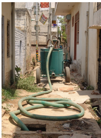
Figure 16: Vacutug in operation
